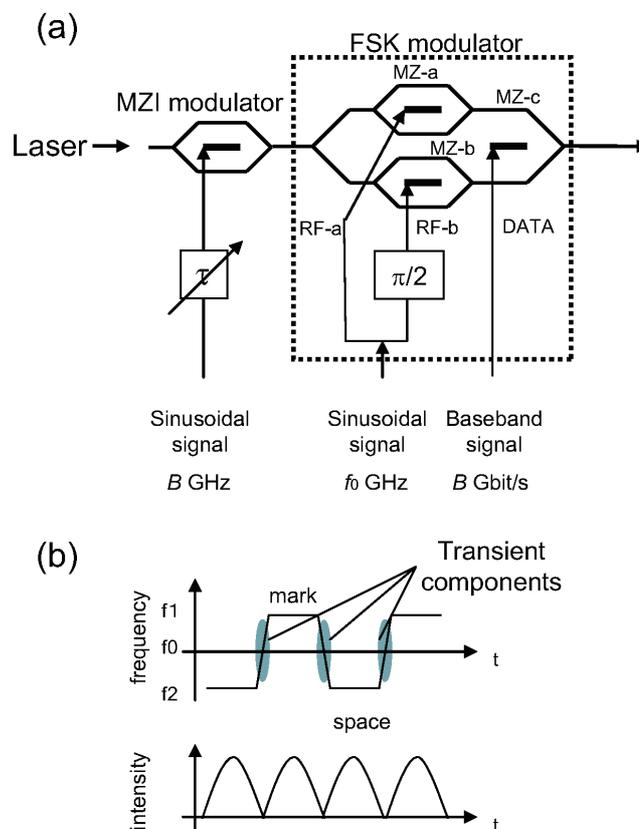
**Fig. 1.** Concept of FSK modulation with a “pulse-carving” technology. (a) Basic structure; (b) suppression of transient components.
