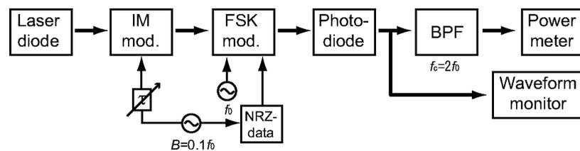
Fig. 2. Simulation model.
