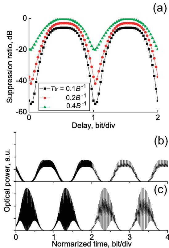
**Fig. 3.** (a) Suppression ratio of the transient components as a function of timing delay of pulse carving signal. Optical waveforms. (b) Timing delay between pulse carving signal and baseband data is in the optimum condition,  $\tau = nB^{-1}$ , and (c) in the worst case,  $\tau = (n + 1/2)B^{-1}$ .
