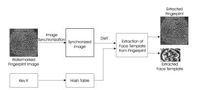
Fig. 2. Watermark Extraction Process
