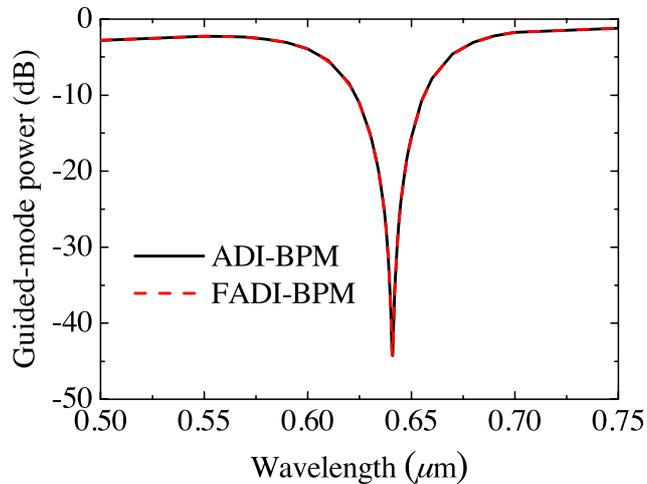
**Fig. 2.** Output guided-mode power versus wavelength. The sensor section is 200 μm in length. The resonance wavelength is around  $\lambda = 0.64 \mu\text{m}$ .
