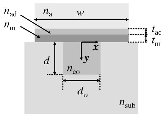
Fig. 1. Configuration of a waveguide-based SPR sensor.
