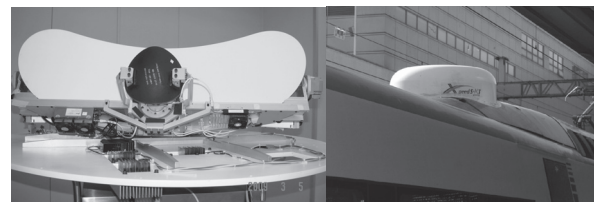
Fig. 6 XpeedSAT low-profile satellite antenna.
