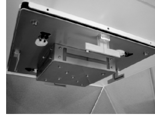
Fig. 12 Photos of the MIMO antenna constructed using four slot and dipole antennas.
