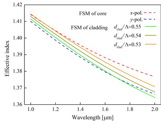
**Fig. 6** Effective indices of the core region and cladding region FSM of the  $x$ SPHF. The dashed curves are the FSMs of the core (red and blue curves indicate the  $x$ - and  $y$ -polarization, respectively) and the solid curves are the FSMs with different cladding hole sizes, from the top to bottom, in order,  $d_{clad} = 0.53\Lambda$ ,  $0.54\Lambda$ , and  $0.55\Lambda$ .
