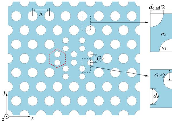
**Fig. 2** Cross section of a  $y$ SPHF with double-hole units in the core. One unit hexagonal cell is represented by red thick dashed frame in which two circular air holes is arranged along the  $y$  direction.
