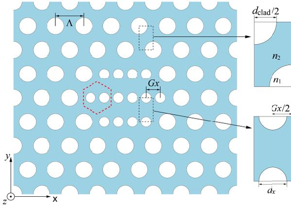
**Fig. 1** Cross section of an  $x$ SPHF with double-hole units in the core. One unit hexagonal cell is represented by red thick dashed frame in which two circular air holes is arranged along the  $x$  direction.
