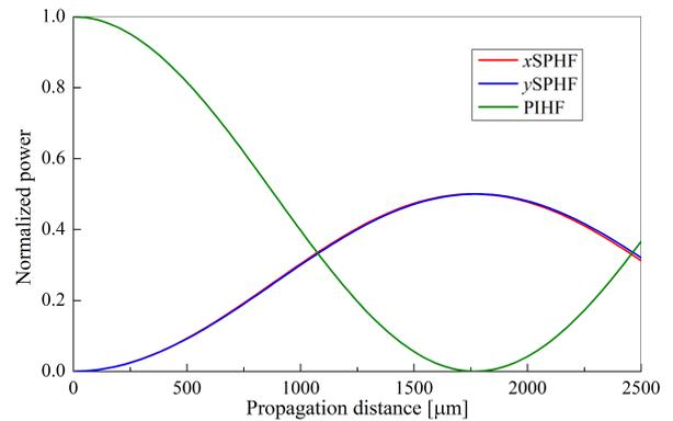
**Fig. 10** Normalized power for the input PIHF and two output SPHF along the propagation distance.
