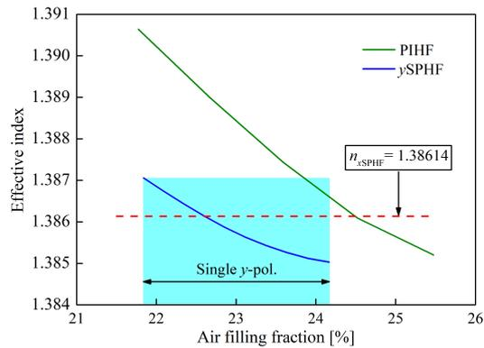
**Fig. 8** Effective refractive indices of waveguides for the  $y$ SPHF and PIHF as a function of air filling fraction at  $\lambda = 1.55 \mu\text{m}$ . The single  $y$ -polarization operation region is the same as in Fig. 7.
