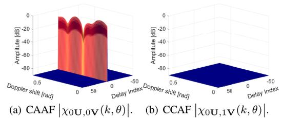
**Fig. 3** CAAF and CCAF based on the generalized null space method.
