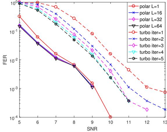
**Fig. 5** Comparison of FER performance of polar codes and turbo equalization with  $T = 1024$ .
