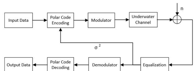
Fig. 1 Block diagram of the system model.
