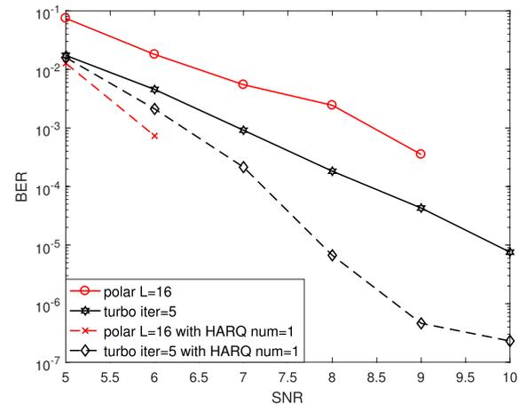
**Fig. 8** BER comparison with/without HARQ mechanism with  $T = 1024$ .
