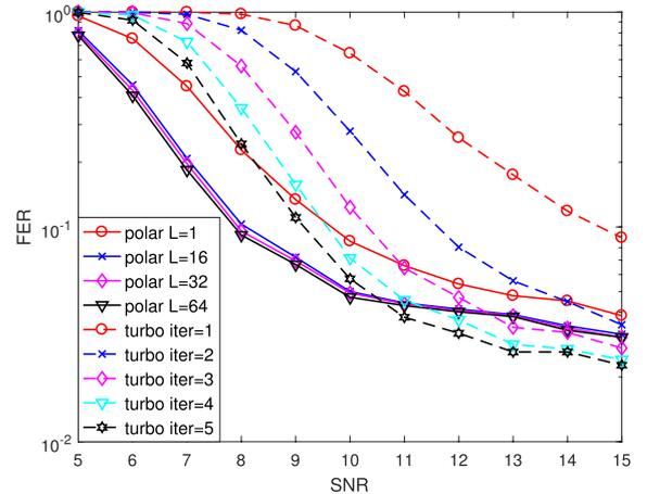
**Fig. 3** Comparison of FER performance of polar codes and turbo equalization with  $T = 512$ .
