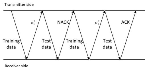
Fig. 2 The proposed HARQ mechanism.
