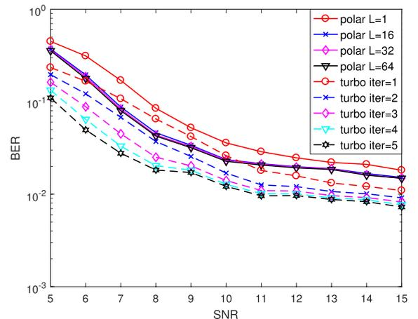
**Fig. 4** Comparison of BER performance of polar codes and turbo equalization with  $T = 512$ .
