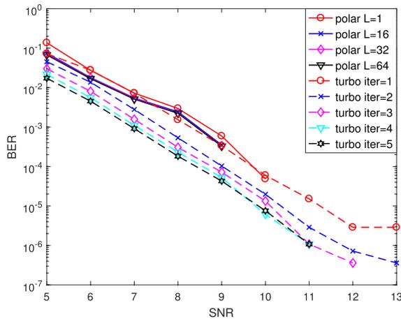
**Fig. 6** Comparison of BER performance of polar codes and turbo equalization with  $T = 1024$ .
