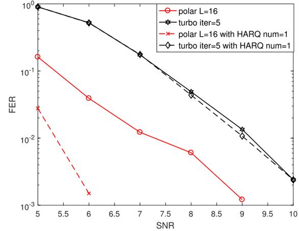
**Fig. 7** FER comparison with/without HARQ mechanism with  $T = 1024$ .
