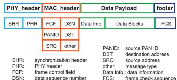
Fig. 1 Packet format for wireless sensor networks.
