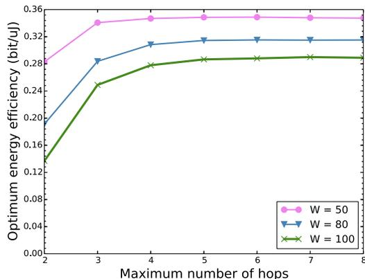
Fig. 10 Optimum energy efficiency with variable maximum number of hops.
