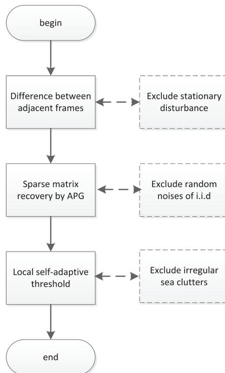
Fig. 2 The flow chart of LRSFD.
