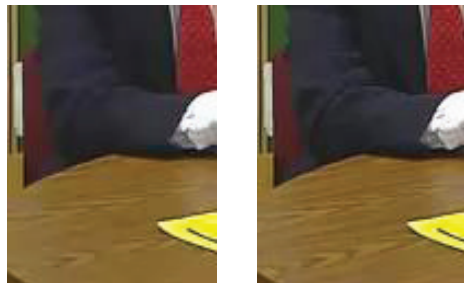
(c) Zoom-in of Area-blue. (Left: fixed-QP, SSIM = 0.8972. Right: CPQ, SSIM = 0.9458)
