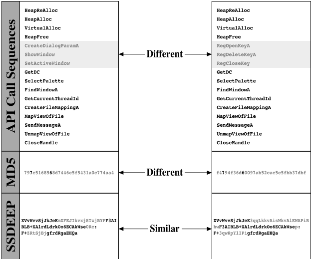
Fig. 5 Comparison of a cryptographic hash and fuzzy hash for API call sequences
