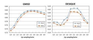
Fig. 3 Impact of up-samping factors on the metric performances.
