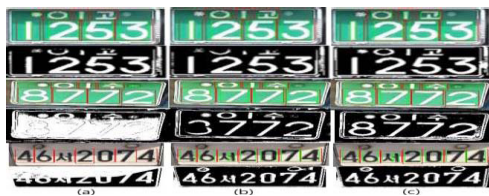
Fig.5 Examples of character detection and binarization results: (a) Otsu's method, (b) improved Bernsen, and (c) proposed method.
