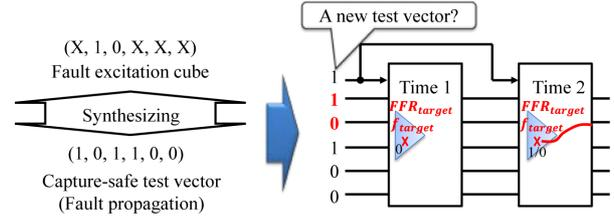
Fig. 8 Test Vector Synthesis
