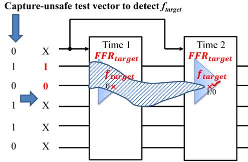
Fig. 6 Example of fault excitation cube extraction
