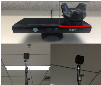
Fig. 1 Hardware system. Top row, the localization sensor (in red box) mounted on a Microsoft Kinect. Bottom row, two base stations.
