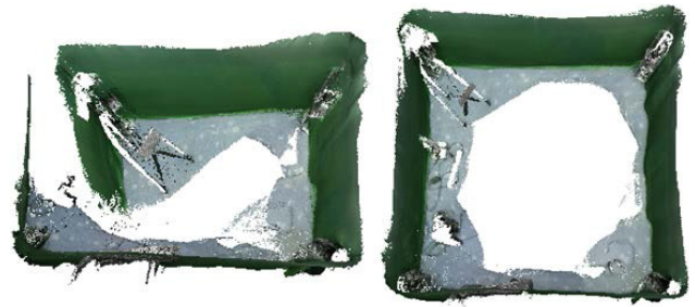
Fig. 4 The comparison of reconstructing a green screen studio. From left to right, results using ElasticFusion [3] and our method.
