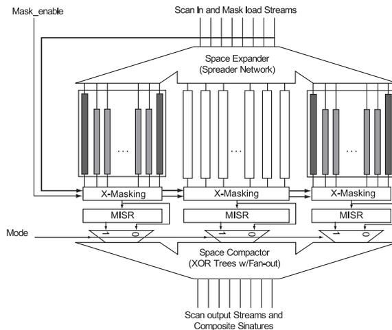
Fig. 1 MISR-based hybrid compression structure.
