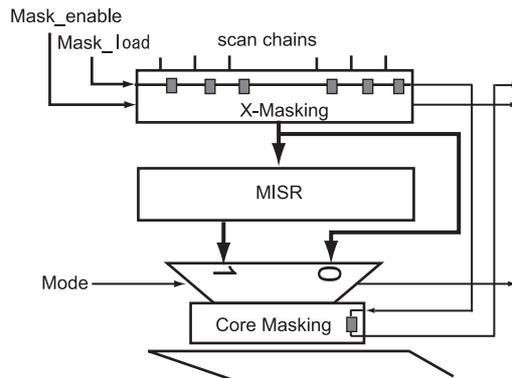
Fig. 3 Compression supporting partial good die.
