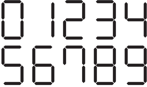
Fig. 3 Number patterns displayed on a seven-segment display.
