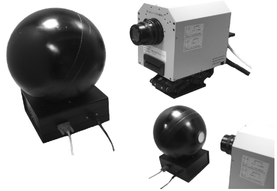
Fig. 4 Accomplished prototype of the XYZ camera with embedded color calibration system based on the LED Color Generator.
