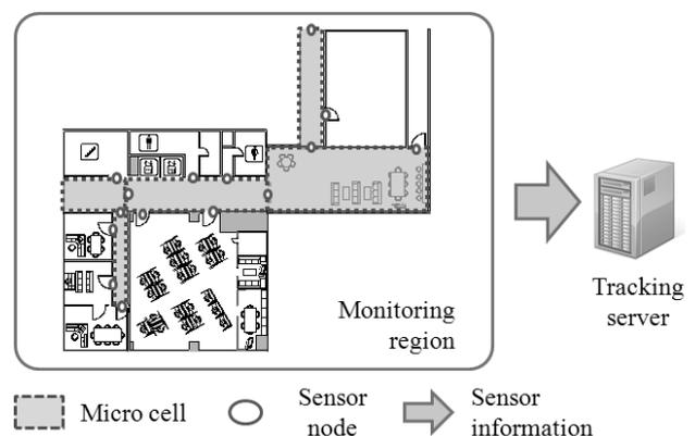
Fig. 1 Object tracking with indoor sensor networks.
