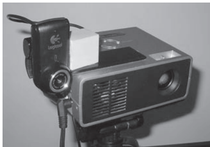
Fig. 11 The rigidly attached handheld projector-camera system.
