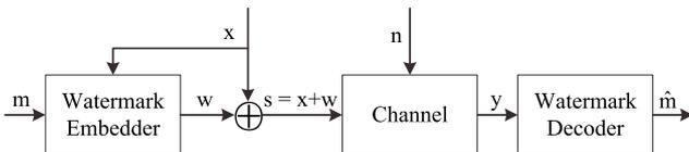
Fig. 1 The communication system model of watermarking with side information.
