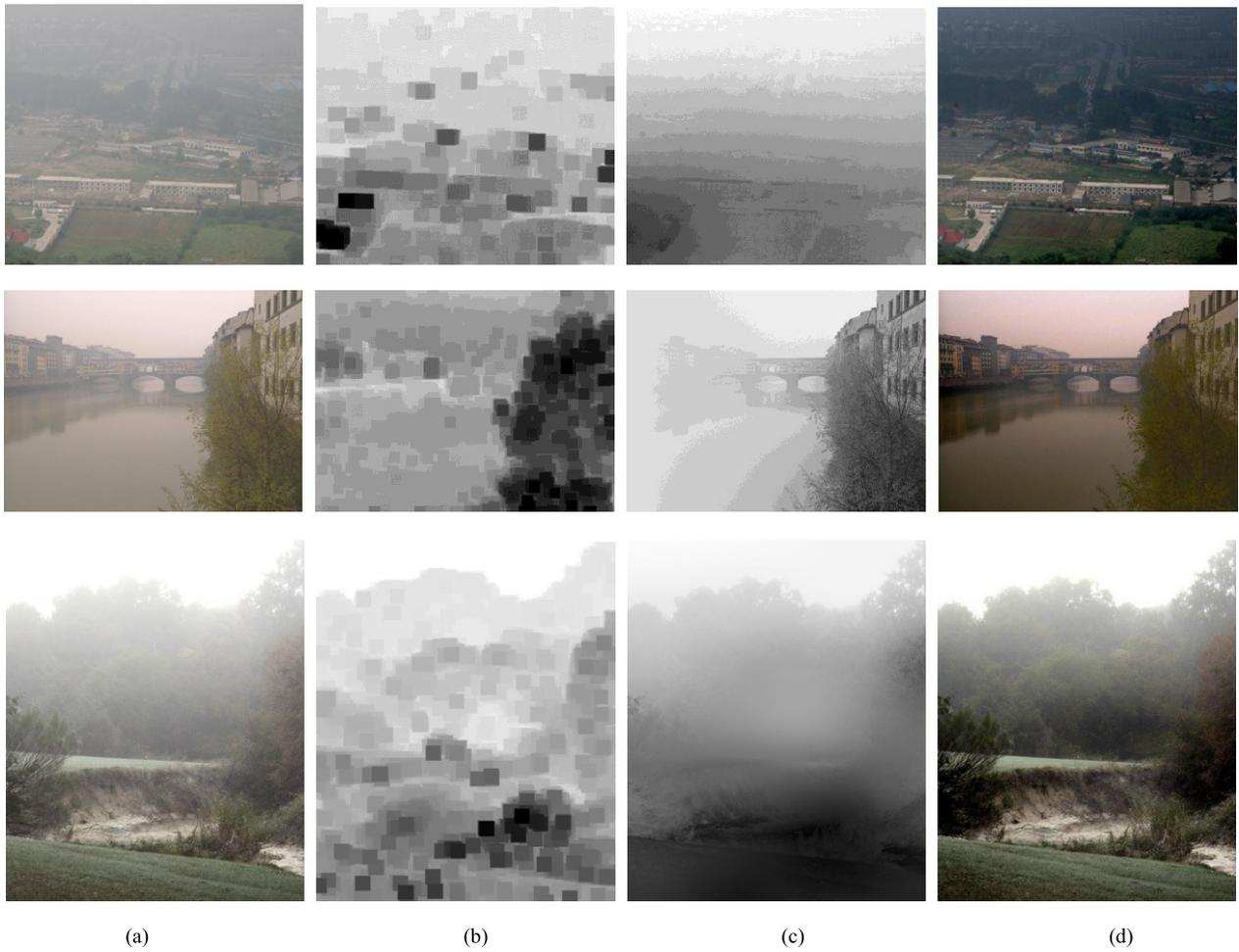
**Fig. 7** De-hazing procedure from foggy image: (a) Foggy images (b) Estimated scene depth from  $d(x)$  (c) Refined scene depth images using guided filter (d) De-hazing results of our approach.
