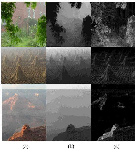
Fig. 4 Relationship between  $Z(x)$  and Relative scene depth: (a) Foggy image, (b) Relative scene depth, (c) Results of  $Z(x)$ .
