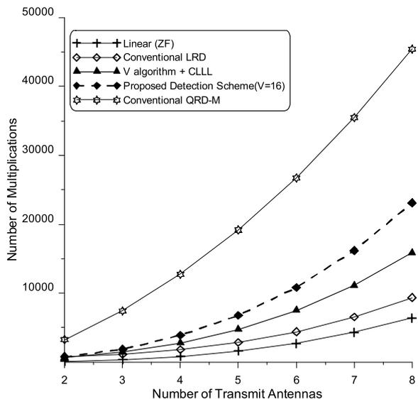
Fig. 2 Complexity of ZF, complex LRD, QRD-M and proposed scheme.
