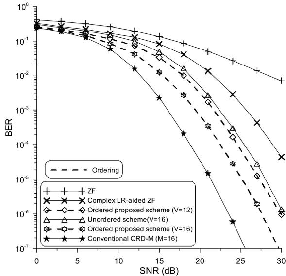
Fig. 1 BER performance of ZF, complex LRD, QRD-M and proposed scheme.
