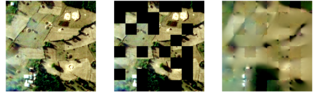
Figure 10: Reconstruction results from the Swin v2 masked autoencoder trained on 150k unlabelled Skysat imagery
