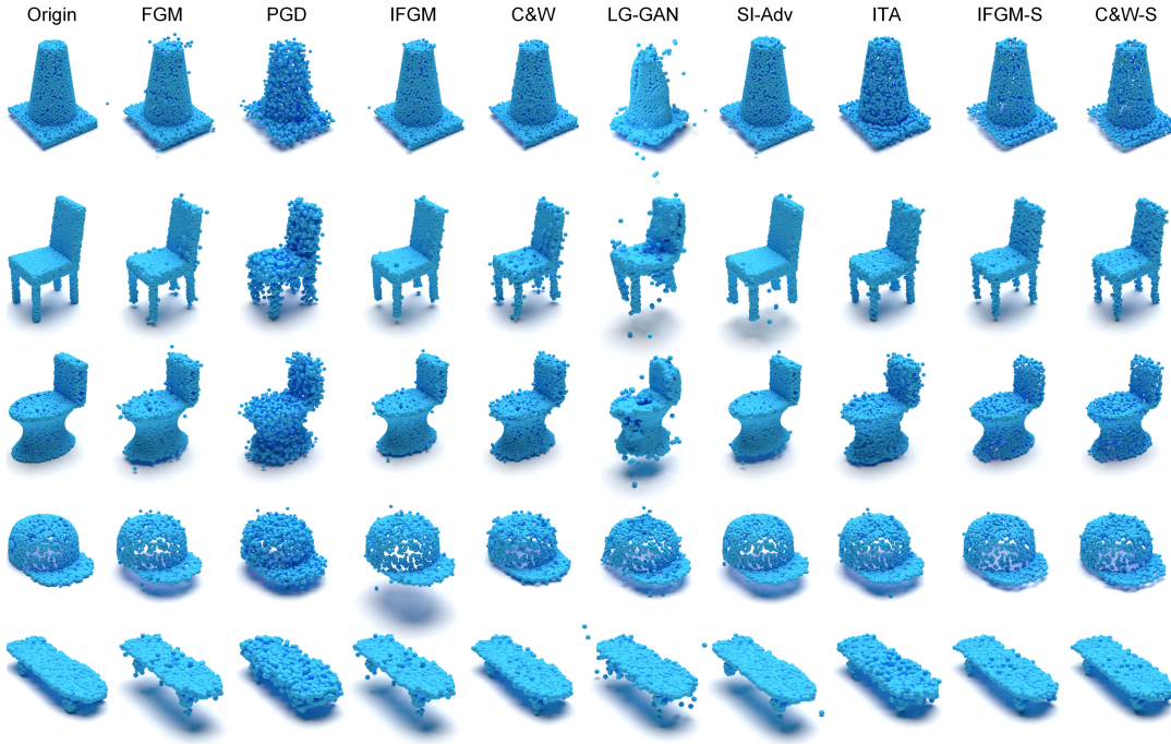
Figure 3: Visualization of original point clouds and the corresponding adversarial point clouds generated by different attack methods for attacking PointNet. The predicted categories before and after attack from top to bottom are: CONE \rightarrow RANGE HOOD; CHAIR \rightarrow TOILET; TOILET \rightarrow CHAIR; CAP \rightarrow LAMP; SKATEBOARD \rightarrow TABLE.
