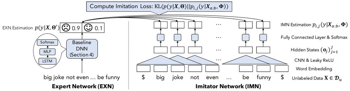
Figure 2: Overview of the 1st IMN ( $c_1 = 1$ ). The IMN must predict the label estimation of the EXN from a limited amount of information. \$ denotes a special token used to pad the input (a zero vector).
