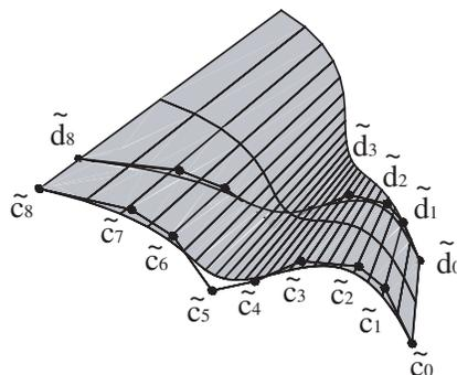
**Fig. 9** Restriction of the developable surface patch in Figure 8
