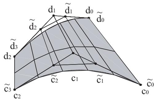
**Fig. 3** Degree-elevated developable surface of one piece of degree 2
