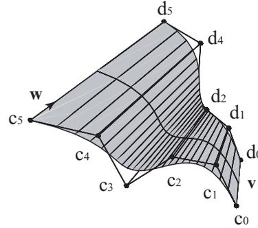
**Fig. 8** Developable surface of degree 3 and 3 pieces
