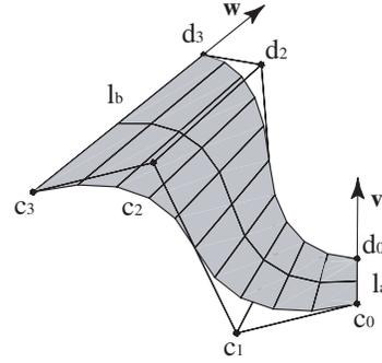
Fig. 4 Developable surface of degree 2 and 2 pieces
