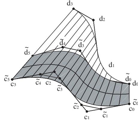
**Fig. 6** Developable surface of degree 2 and 2 pieces stretched to a patch of degree 3
