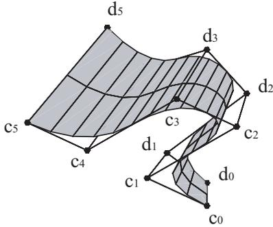
**Fig. 2** Developable B-spline surface of 4 pieces of degree 2
