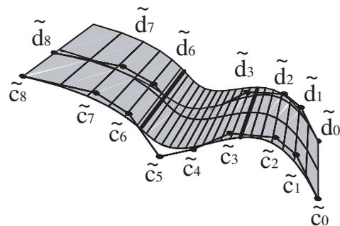
**Fig. 7** Degree-elevation and restriction of the developable surface patch in Figure 5
