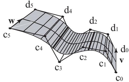
**Fig. 5** Developable surface of degree 3 and 3 pieces
