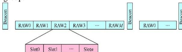
**Figure 1.** Principle of RAW for beacon transmission
