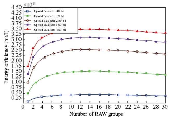
**Figure 4.** The Impact of Data Packet Size on the energy efficiency
