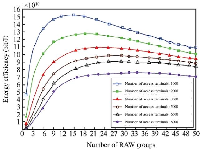
**Figure 5.** The impact of the total number of terminals on system energy efficiency
