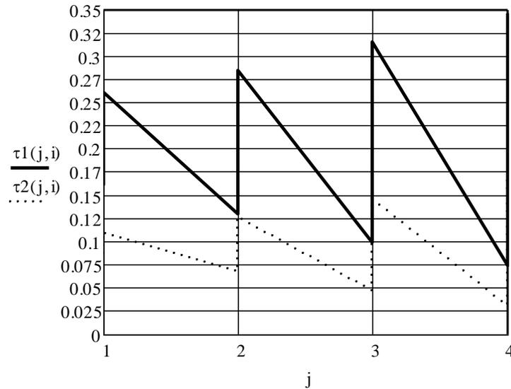
**Figure 4.** Dependence of packet time delays on changes in packet intensities and lengths when using communication channels with different bandwidths ( $\tau_1$  at  $V_k = 128$  Kbps,  $\tau_2$  at  $V_k = 192$  Kbps).
