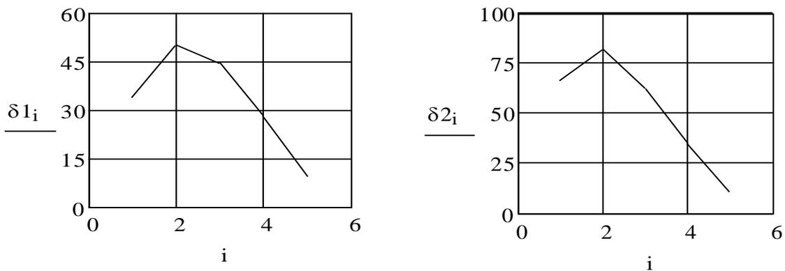
**Figure 5.** Dependence of the effect (%) of channel bandwidth utilization on the coefficient (k) with packet delay constraints of 150 ms ( $\delta 1$ ) and 300 ms ( $\delta 2$ )
