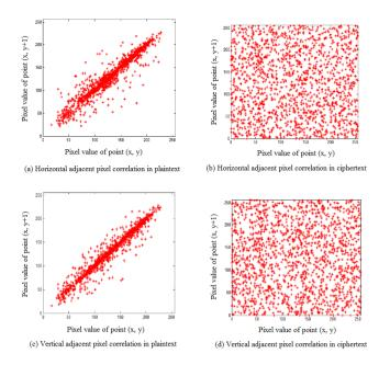
Figure 6. Correlation of horizontal and vertical adjacent pixels before and after encryption
