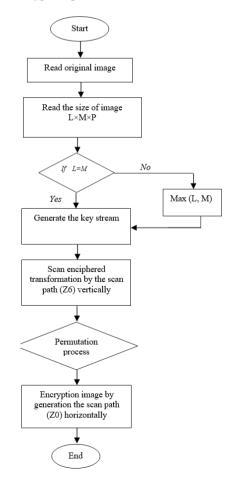
Figure 6. Flow Chart of encryption process
