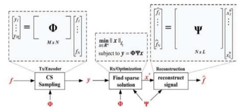
Figure 6. Function of compression sampling technique
