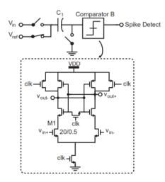
Figure 4. Schematic spike detector circuit with spike output in the technology of 180 nm
