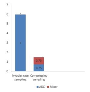
Figure 8. Comparison of power consumption of compressive sampling and sampling at Nyquist rate
