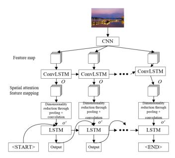
Figure 2. The extraction of spatiotemporal features based on ConvLSTM and spatial attention
