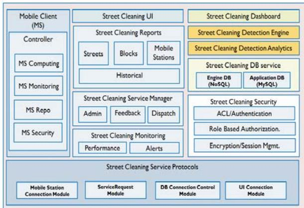
Fig.7 High-level Architecture
