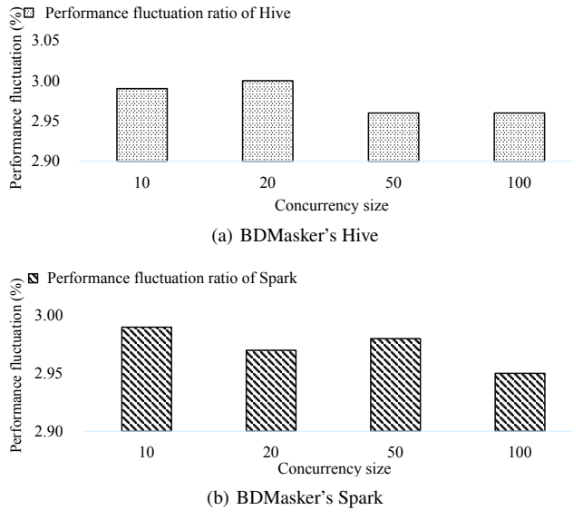
Figure 14 Performance fluctuations of dynamic masking of BDMasker's SQL engines in multi-concurrency scenarios
