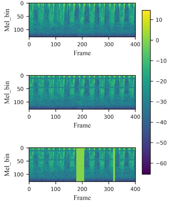
Figure 2. Spectrogram augmentation. Top: original Mel-spectrogram, Middle: Mel-spectrogram after masking in frequency domain, Bottom: Mel-spectrogram after masking in time and frequency domain
