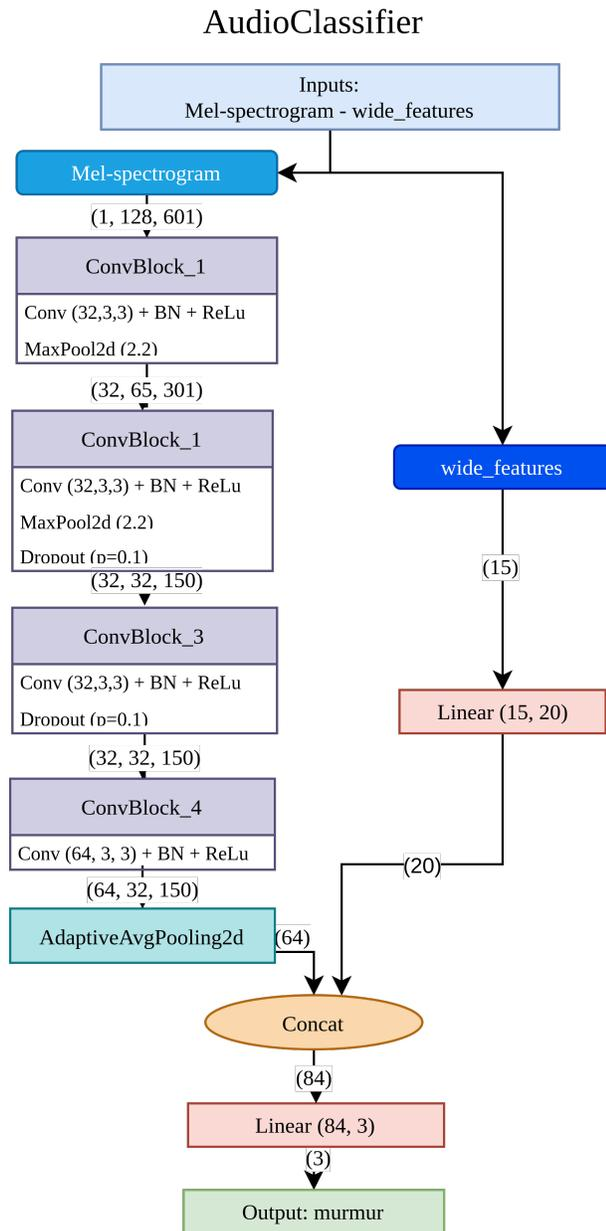
Figure 3. Illustration of the proposed model structure. The network uses the Mel-spectrogram and the wide features as inputs and returns as outputs the heart murmurs classification.
