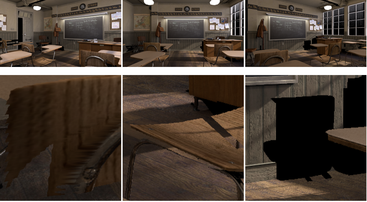
Figure 2. Classroom dataset. Top row: Synthesized views using 4 input views and rotating around a central point in the scene. Bottom row: Zoomed in details of a bad blending (hardly visible at full scale), a small disocclusion and a full disocclusion. All three problems are due to missing information (i.e. information not captured by any camera).
