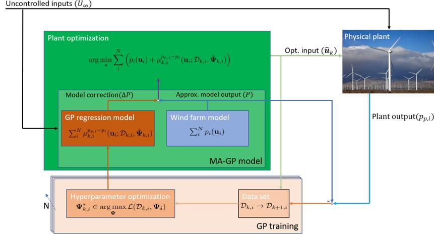
Fig. 1: The basic idea of the distributed MA-GP scheme for a wind farm <sup>1</sup>.
