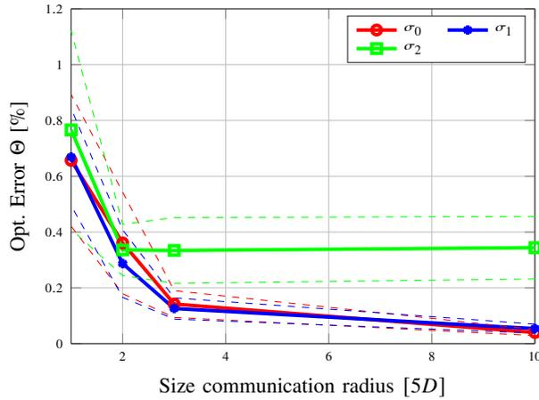
(c) Influence of communication radius on the optimization error with an initial training set size of 600 data points. The x-axis indicates of how many upwind turbines the control inputs are used in the learning of the individual GPs.
