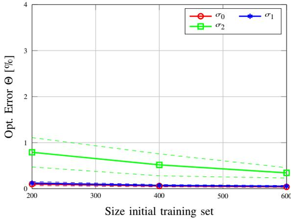
(a) Distributed learning approach with different noise levels. The solid line show the mean and the dashed lines the standard deviation of the error of the 20 test runs.
