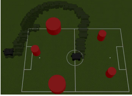
Fig. 8. Gazebo simulation considering the Neobotix MPO-500. Three out of five obstacles are known.
