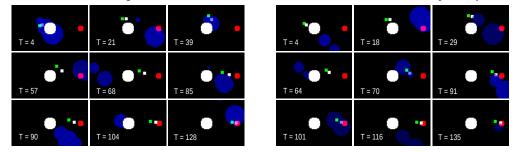
Fig. 6: Snapshots of the trajectories of the robots implementing the hybrid controller, but using different perception maps. In the left figure, the perception map was trained on images *without* occlusions (shown in blue color). In the right plot, the perception map was trained using images *with* occlusion. In both cases, the hybrid controller is successful.
