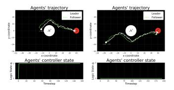
Fig. 7: Performance of the controllers when noise ( $\epsilon \sim \mathcal{N}(0, 0.5)$ ) is added to the states of the robot, and the sensor of the follower has a failure rate of 50% (no photo is taken). The flow and jump sets for this controllers are defined with  $\chi = 1.1$  and  $\lambda = 0.09$ .
