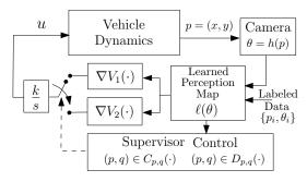
Fig. 4: Scheme of the closed-loop system.
