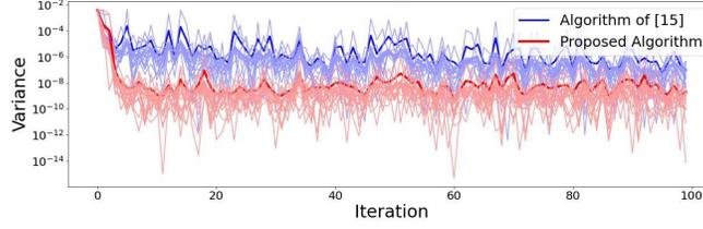
Fig. 7: Variance of cost function for the second case ( $S = 10$  and  $M = 5$ ) over 20 Monte Carlo iterations (thicker line correspond to the mean of Monte Carlo iterations,  $y$  axis is limited for the purpose of better visualization).
