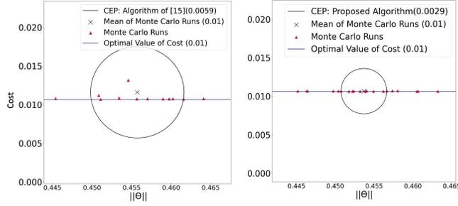
Fig. 5: CEP graph for the second case ( $S = 5$  and  $M = 2$ ) over 20 Monte Carlo iterations. The results for our algorithm is in the right while the result for algorithm of [15] is shown on the left.
