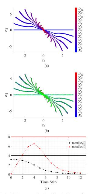
Fig. 3: (a) Over-approximation of reachable sets of nonlinear system (12) in closed-loop with saturated LQR (13). (b) Closed-loop trajectories of the nonlinear system from a random sampling of initial conditions within  $\mathcal{X}_0$ , plotted over the over-approximations of forward reachable sets. (c) Maximum magnitudes of  $x_1$  and  $x_2$  plotted for each time step. Solid lines with matching colors correspond to  $D(\Phi)$ in the  $x_1$  and  $x_2$  dimensions.
