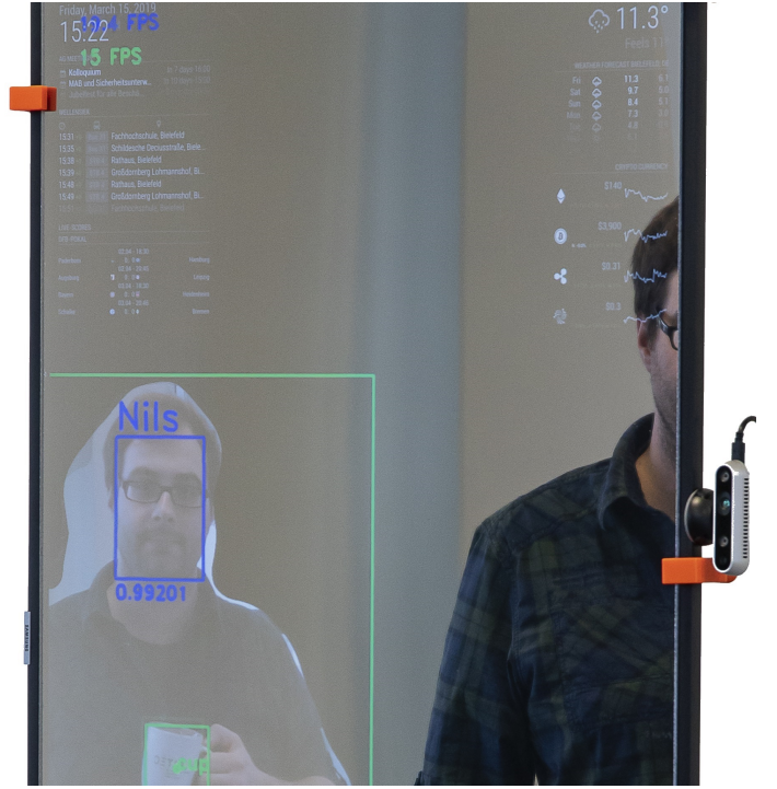
Fig. 8: User interface and interaction with the Smart Mirror.
