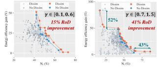
Fig. 7. Inner optimization improvement by regularizing the exits scores with the dissimilarity function  $(dissim)^{\gamma}$  over two ranges of  $\gamma$  values
