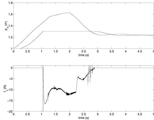
Figure 5: Interaction with an obstacle ( $p_x = 1.3$ ): master (solid) and slave (dashed) along  $x$  direction and force applied to the environment at the slave side.
