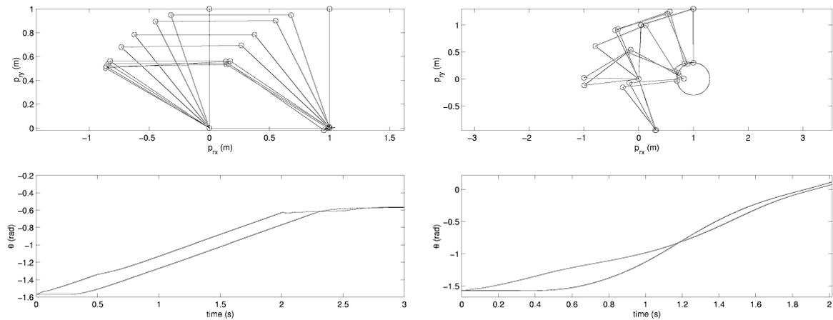
Figure 6: [Left] Screwing a bolt ( $P_x = 1$ ,  $P_y = 0$ ): master (solid) and slave (dashed) motion and end effector orientation  $P_\theta$ . [Right] Turning a grip handle ( $(x - 1)^2 + y^2 = 0.3^2$ , with the last link perpendicular to the trajectory): master and slave motion and orientation.
