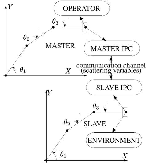
Figure 1: Telemanipulation control scheme.
