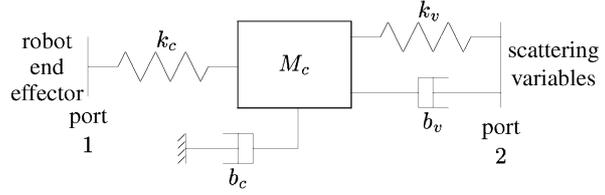
Figure 2: Physical interpretation of an intrinsically passive controller (master and slave IPC).
