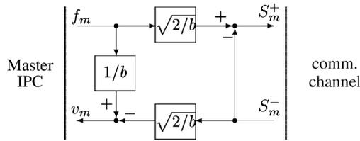
Figure 3: Scattering transformation at the master side.
