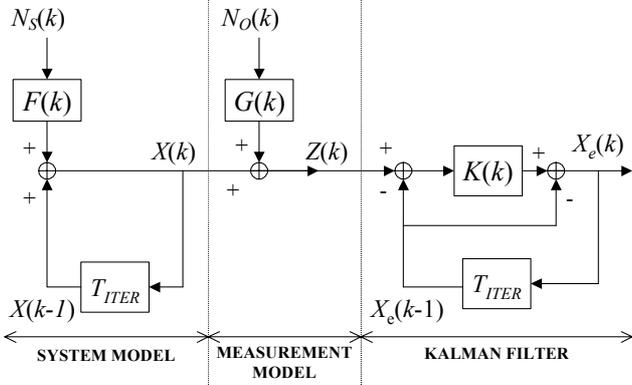
Fig. 2: System model, measurement model and Kalman filter
