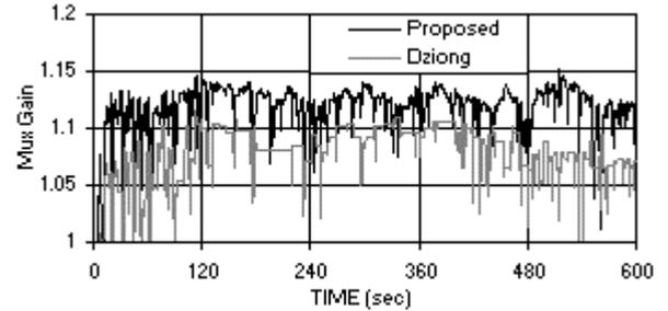
Fig. 5: Multiplexing (Mux) Gain for IRM and Dziong
