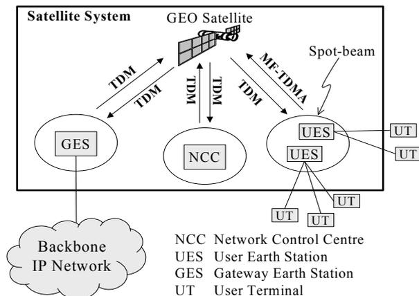
Fig.1 : Reference Satellite System scenario
