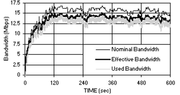
Fig. 3: Used, Nominal and Effective Bandwidth in the solution proposed in this paper
