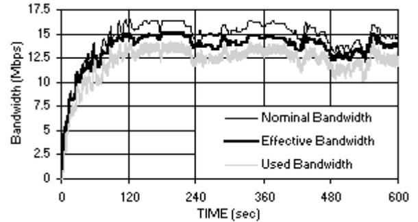
Fig. 4: Used, Nominal and Effective Bandwidth in the solution proposed in [8]
