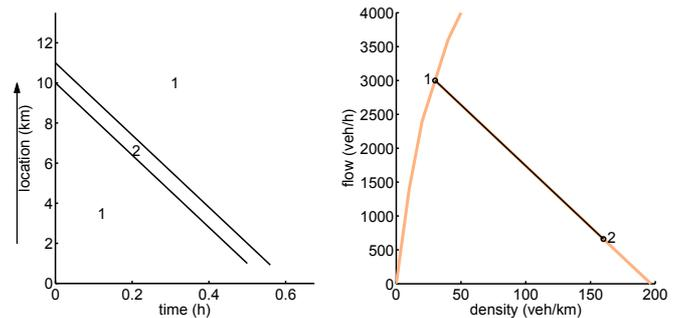
Fig. 1. According to the shock wave theory the propagation of the front between two traffic states (left figure) has the same slope as the line connecting the two states in the density-flow diagram (right figure). The arrow indicates the travel direction.
