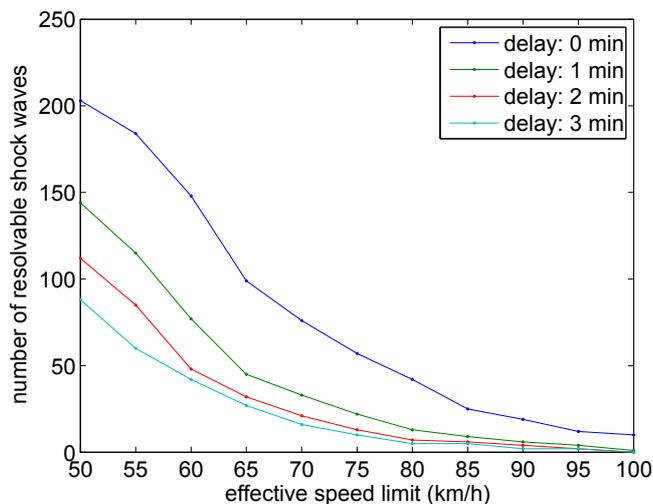
Fig. 4. The number of solvable shock waves (out of 407) as a function of the effective speed limit for various measurement delays.
