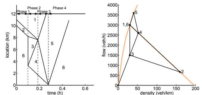
Fig. 2. The four phases of the SPECIALIST algorithm. Phase 1: The shock wave is detected. Phase 2: Speed limits are turned on in areas 2, 3, and 4. The shock wave dissolves. Phase 3: The speed-limited area (area 4) resolves and flows out efficiently. Phase 4: The remaining area 5 is a forward propagating high-speed high-flow wave.
