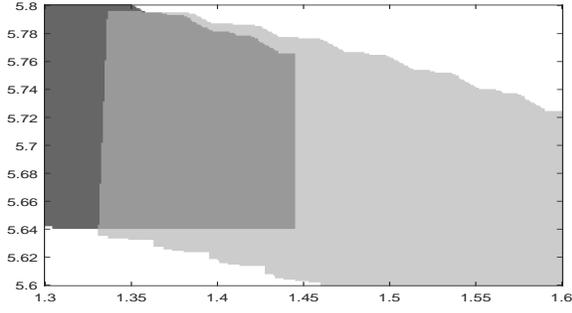
Fig. 1. Safety controller designed for a symbolic model of the boost DC-DC converter with a fixed time sampling period  $\tau^* = 0.5\text{sec}$  (dark gray: mode 1, light gray: mode 2, medium gray: both modes are acceptable, white: uncontrollable states).
