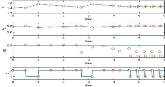
Fig. 3. Evolution of the state variables of the boost DC-DC converter with the lazy safety controller starting at  $x = [1.45, 5.77]^T$ ; The sampling instants generated while computing the lazy safety controller; Switching signal generated by the lazy safety controller
