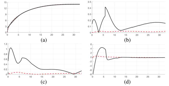
Fig. 2. Simulation results for the first scenario (dashed red lines), second scenario (dash-dotted blue lines), and third scenario (solid black lines). a) Resulting position on the vertical plane:  $-\bar{Z}$  v.s.  $\bar{\mathbf{X}}$ , b) norm of the output  $y = [\tilde{x} \ \tilde{z}]^T$ :  $\|y\|$  v.s.  $\bar{\mathbf{X}}$ , c) norm of the time derivative of the output:  $\|dy/dt\|$  v.s.  $\bar{\mathbf{X}}$ , and d) incremental pitch angle:  $\theta$  v.s.  $\bar{\mathbf{X}}$ .
